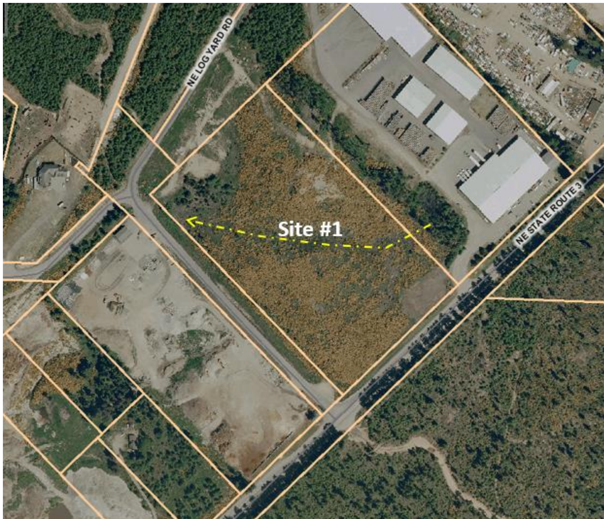
Figure 2. Site #1: yellow line shows location of swale crossing which might conduct overflow water from the stormwater facility on adjacent parcel to N.
